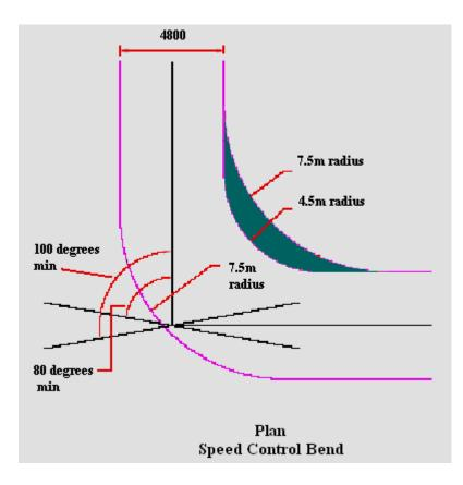
Figure 3.9 Speed Control at a bend
