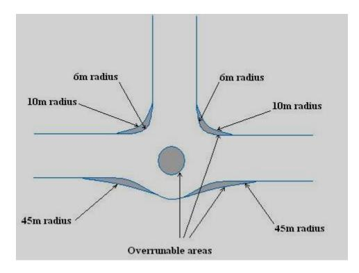
Figure 3.11 Speed Control at a Roundabout
