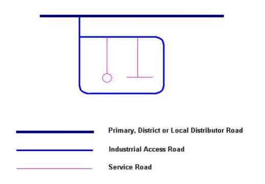
Figure 4.1 Diagrammatic layouts for industrial trading estate roads
