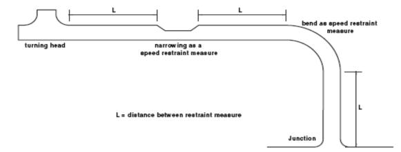
Figure 3.7 Speed Control restraints
